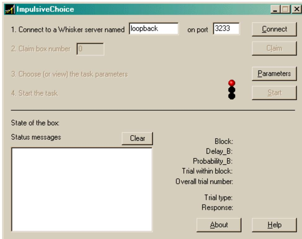
You must connect to a Whisker server, claim an operant chamber (box), and set up the [parameters](#) for your task. Once that's done, the traffic lights will turn amber. When you are ready, press *Start* to begin the task. When the task is running, it looks like this:
